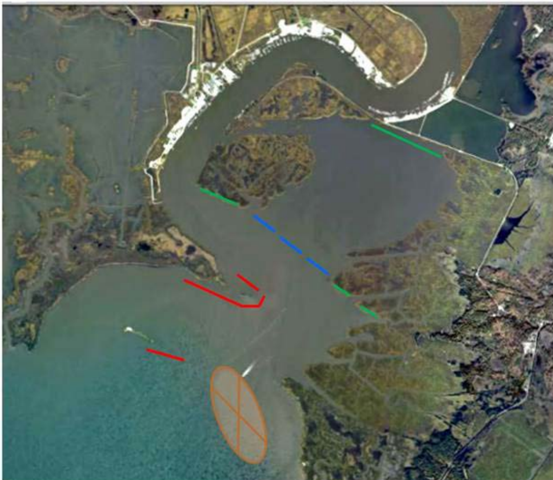
Figure 14: Conceptual example of a hybrid strategy for stabilizing an eroding tributary shoreline.
